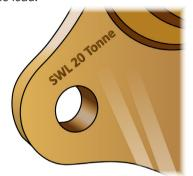
2. If your loader has a lifting lug on the bucket, connect to the lug. If not, fit a iib attachment and use it.
