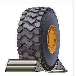
15. Use chains to safely secure the front end loader to the transport vehicle. Remove and stow chocks when the machine is secured.
