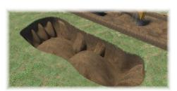
The excavator or dozer may use material from the borrow pit to build up low areas in the road. They may also build up diversion blocks. Diversion blocks divert water away from the road and into drains.
