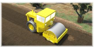
A site supervisor or roller operator tests the compaction. Sometimes they will use a deflectometer or penetrometer. Some rollers/compactors can test the compaction as they drive.
