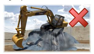
Keep filling out the stockpile one row at a time or by dozing material to the correct position on the stockpile.
