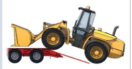
7. As the machine rocks over onto the deck, raise the bucket slowly to prevent the machine coming down hard onto the deck.
