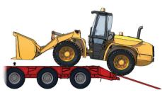
8. Raise the bucket to just clear the deck and position the machine on the vehicle to make sure the load is correctly shared by the wheels.
