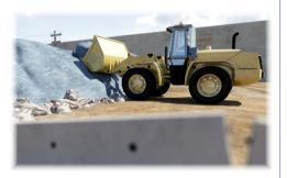
2. Try not to fill too close to the edge. The edge of the stockpile could give way.
