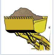
Put a layer of soil in the truck before dumping large rocks
